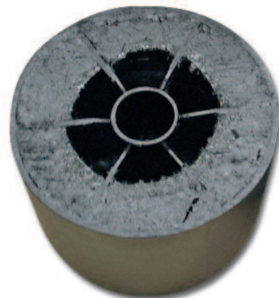
Sectioned Rotor with Contaminant
